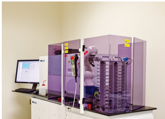
The PerkinElmer Opera microscope allows investigators to automatically capture hundreds of thousands of images in a few hours.
